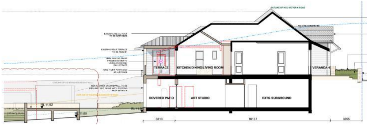
Figure 12: Proposed long section – Dwelling 1 (ground floor) and Dwelling 3 (lower ground floor)
